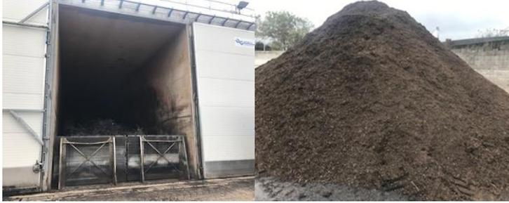
The process would involve reception of waste in a sealed negative pressure building, shredding and mixing of waste, then storage of waste in an enclosed composting tunnel before being transferred to an outdoor aerated static pile composting facility for stabilisation/maturation and then screening. Any unsuitable material would be sent off site to be re-processed into a biomass fuel for energy and/or heat recovery.
